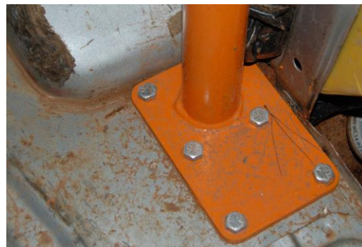
Fig 7 – Upper C pillar mounting plate orientation
