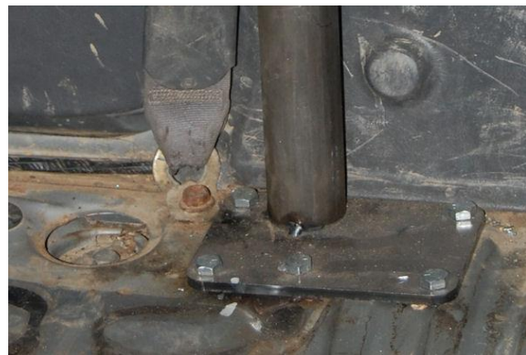
Fig 5 – Upper B pillar mounting plate orientation
