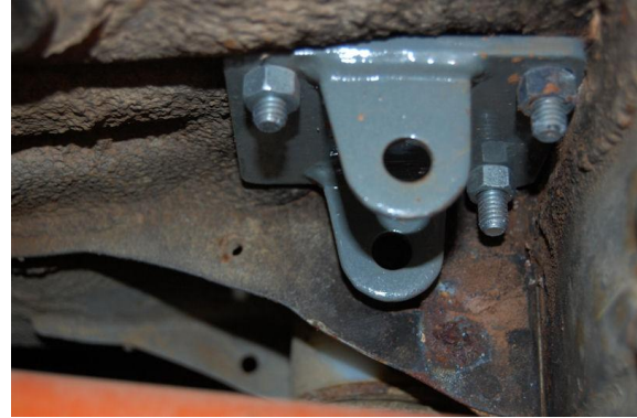
Fig 4 – A pillar lower foot alignment
