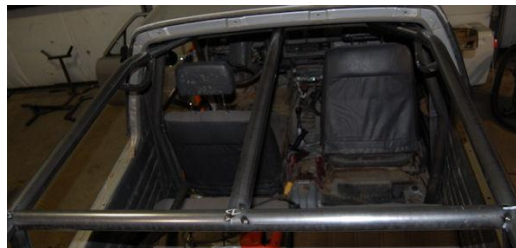
Fig 11 – 5RIC Rear Half being installed.
