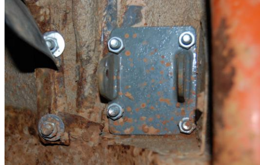
Fig 8 – Lower C pillar mounting plate orientation
