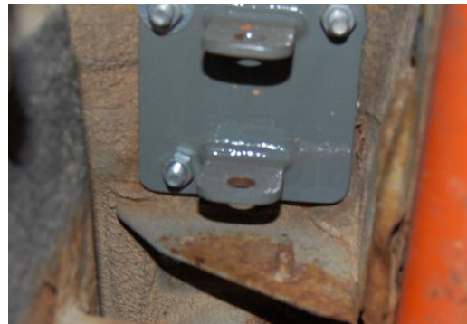
Fig 6 – Lower B pillar mounting plate orientation
